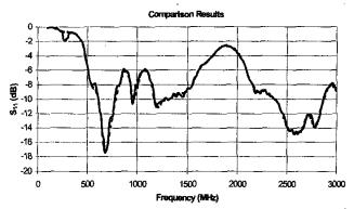
Figure 8b. The  $S_{11}$  values from measurements (solid line) and the output of the neural network (dashed line) for the antenna configuration shown in Figure 7b.
