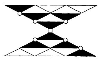
Figure 7b. The reconfigurable antenna structure: The ON switch positions are marked with small circles, and the corresponding activated array elements are shaded black.
