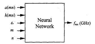
Figure 4. The resonant-frequency calculation of a triangular microstrip antenna using neural networks. A  $5 \times 5 \times 3 \times 1$  multilayer perceptron, trained using a back-propagation algorithm, was used.
