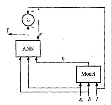
Figure 5. The calculation paradigm for the design of a square patch antenna.  $\varepsilon_r$  is the dielectric constant, l is the side length of the patch,  $\hat{l}$  is the output of the ANN, and Wolf and Knoppik's model for a square patch was used.
