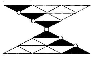
Figure 7a. The reconfigurable antenna structure: The ON switch positions are marked with small circles, and the corresponding activated array elements are shaded black.
