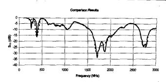
Figure 8a. The  $S_{11}$  values from measurements (solid line) and the output of the neural network (dashed line) for the antenna configuration shown in Figure 7a.
