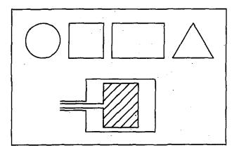
Figure 3. Low-profile antennas considered to date for neuralnetwork applications. Microstrip structures include circular, square, rectangular, and triangular; coplanar waveguide patch/slot antennas.
